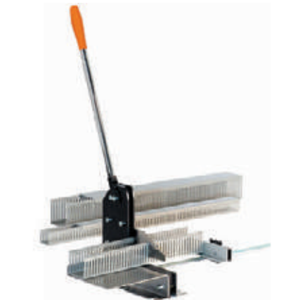
Manually-operated wire channel cutter for cutting wire channels and covers up to a width of 125 mm. • Cutting with no burrs or waste • Longitudinal stop (1000 mm) with guide for precision angling • Table-top unit for mounting on workbench or similar workplaces • Hardened cutting edges made from special steel
