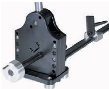
TS 35/7.5 mm according to EN 50022 (s = 1.0 mm)
